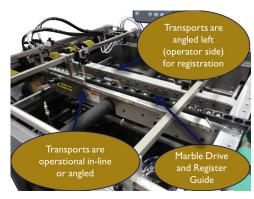
Alignment System and Pre-Breaking Device
