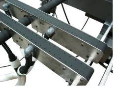
Interchangeable Vacuum Transports The vacuum transports feature Kluge's "drop-in" interchangeable design for fast and easy positioning and removal for off-line maintenance. Vacuum transports are interchangeable with bearing bed transports and eliminate the need for top drive wheel sets and belts allowing for accessories such as ink-jet addressing and variable data systems, vision and verification systems, complex tip-on applications, and label applications.
