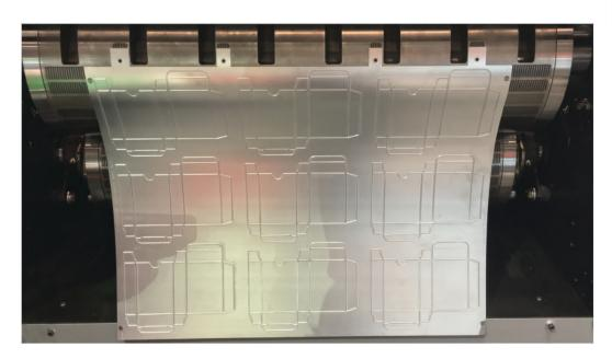
PICTURED ABOVE IS A MALE/FEMALE PAIRED SET OF DIE TOOLS BEING MOUNTED VIA A PIN MOUNT SYSTEM TO ENSURE CORRECT ALIGNMENT. DUAL MAGNETIC CYLINDERS ALSO INCLUDE MICRO-ADJUSTMENTS IN THE MACHINE TO ALLOW FOR VERY FINE TUNING OF THE DIES TO MATCH UP.
